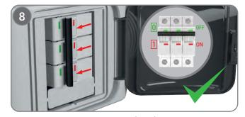
Switch miniature circuit breaker (MCB) to "ON" position and close the transparent cover.
